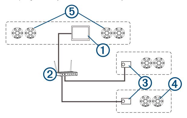
In the image above, one Vieo RV 850 stereo ① connects to a wireless router ② and to two Apollo SRX400 zone stereos ③. The two Fusion PartyBus stereo zone stereos can stream sources from the Fusion PartyBus stereo.
